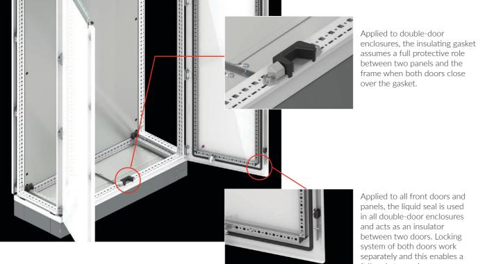
Applied to all front doors and panels, the liquid seal is used in all double-door enclosures and acts as an insulator between two doors. Locking system of both doors work separately and this enables a full gasket pressing
