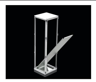
Manufactured from a 3,00 mm galvanized steel, TEOS mounting plates are railed and easily mounted. With its thick steel sheet structure, the mounting plate can carry heavy equipment with its rigid structure and does not need additional side support parts. In this way, bayed enclosure space is increased in combined enclosures.
