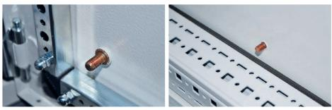
Placed on the aliminium corner combination. the earthing hooks are tightly mounted on the uncoated inner surface of the rails by means of eroding. Thereby, the earthing continuity is ensured for all rails and their parts
