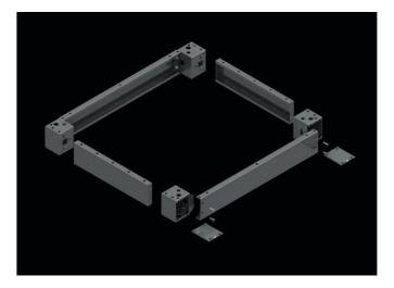
• Neo Modular and Neo monoblock frame system are same as Teos frame related with the bottom dimensions. Therefore plinth system of TEOS which includes H100mm and H200mm version can adapte to Neo Modular and Neo monoblock design.
